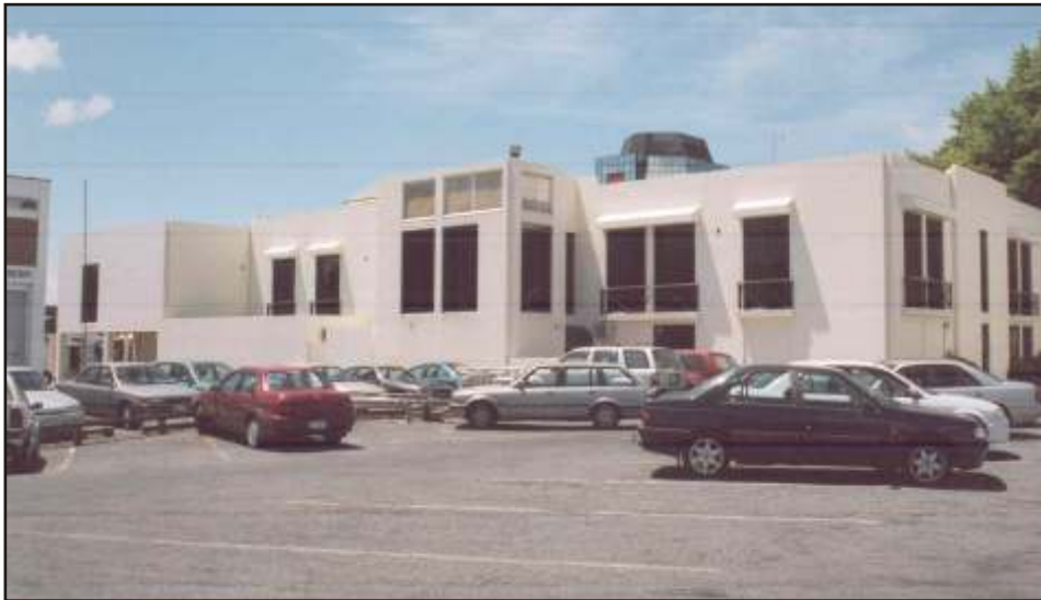
😊 Windows at the rear of the building result in surveillance of the carpark
